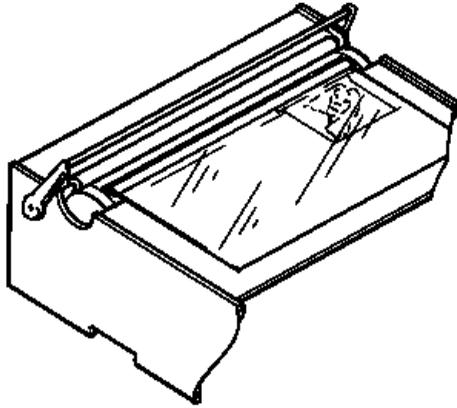
5. Move the padded roller forward to contact the drum.
