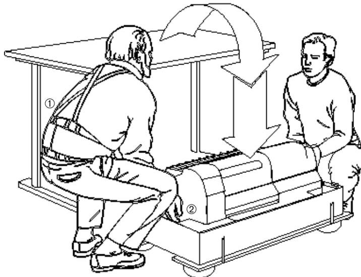
7. Cover the scanner with the poly bag and foam supports.
