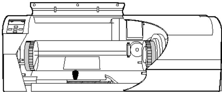
5. Move the drum mounting lever to the closed position and make sure the alignment pin has engaged the drum endcap.
