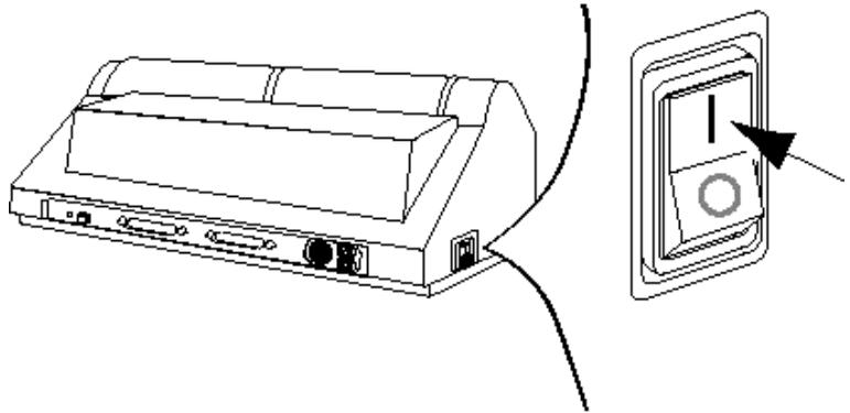
During power-up the HiResolve performs extensive internal diagnostics prior to going on-line. Once the scanner reaches on-line status the control panel displays the message READY TO SCAN). It takes approximately five minutes for the scanner to warm up and stabilize, but the scanner can be used as soon as the message ON LINE appears on the control panel.
