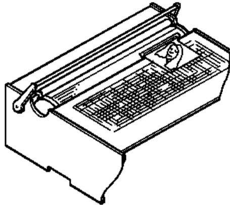
3. Place a sheet of mylar over the image. Use a piece of mylar that extends at least 1/2" (12 mm) past the transparency on all sides.
