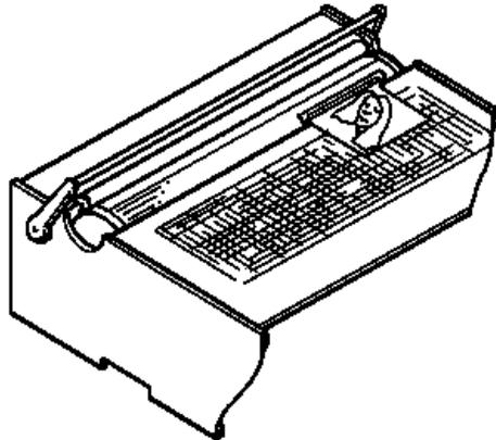
3. Place tape along the edge of the original that is in contact with the drum.
