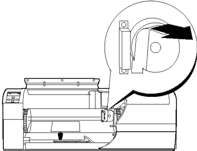
5. Remove the white plastic cover on one of the two SCSI ports, located on the right rear of the scanner. Place the cover in the large resealable bag containing the power cord.
