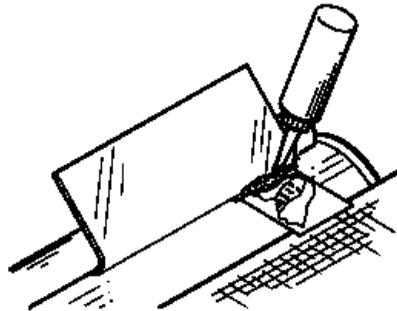
7. Grasp the ends of the drum and turn to the edge of the transparency to press out all the air and any excess oil:
