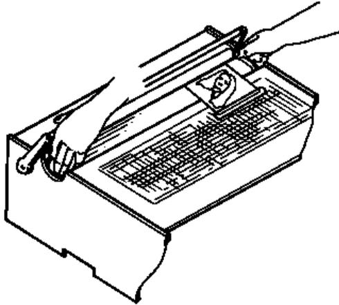
5. With slight pressure applied to the handle, tape the lower edge of the original to the drum.
