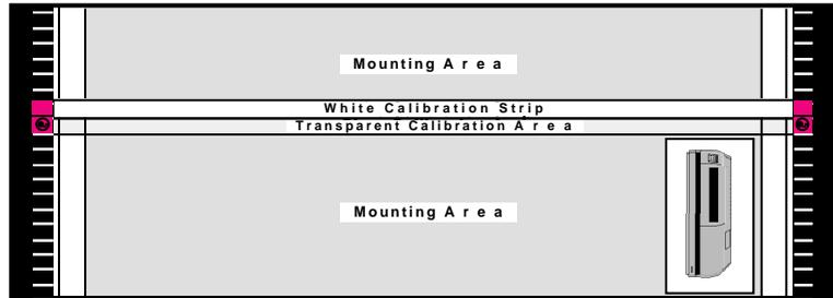
The Howtek HiResolve is designed to maximize the speed of the scan, based on size, position on the drum, and selected magnification of the mounted original. Typically, best performance is achieved when the image is located nearest the upper right-hand side of the drum (as installed) with the long edge of the original parallel to the circumferential scribe lines.
