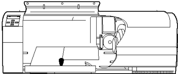
3. Set the drum into the scanner cavity.
