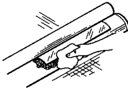
9. Tape the bottom of the mylar sheet to the drum.
