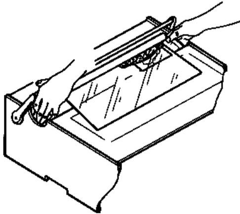
8. Wipe away any excess oil, using a soft cloth and drum cleaner. This will ensure that the tape sticks to the drum:
