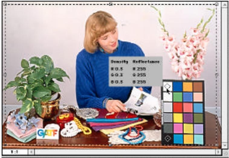
When you select the probe tool, activate a region and move it over the Sticky Densitometer. A window will appear displaying the values for that point.
